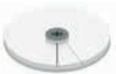
Wider angle between orientation lines produces less deflection.
