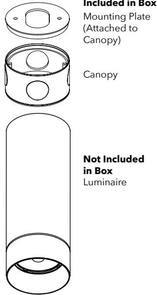
**Step 1.** Unscrew Mounting Plate from canopy and attach to ceiling (Fig. 1).
