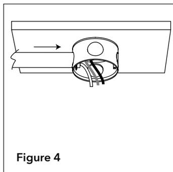
**Step 5.** Pass wires from conduit through canopy and connect to luminaire, following Wire Connections table (Fig. 5).
