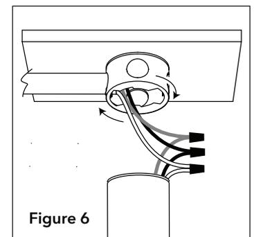
**Step 7.** Conceal wires in canopy. Screw luminaire into canopy by turning clockwise (Fig. 7).
